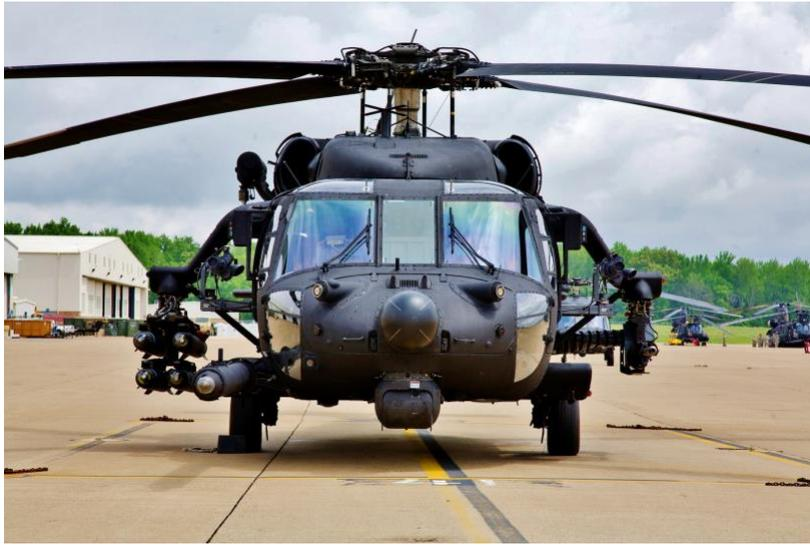
MH-60 Black Hawk helicopter armed with Unitech's Lightweight Armament Support Structure (LASS) weapons pylon.
